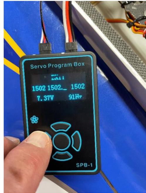
This is now a direct feed from TX or FBL system, used to verify /test changes. **Press top button** to EXIT and go back to home screen.
